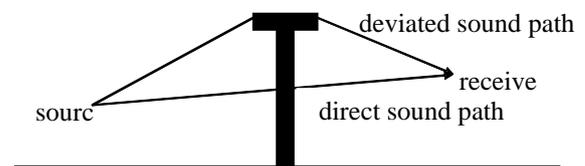
Fig. 6. Direct and deviated sound path with two edges
