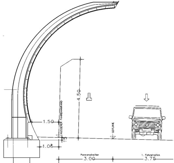
**Fig. 3.** High and curved noise barrier
