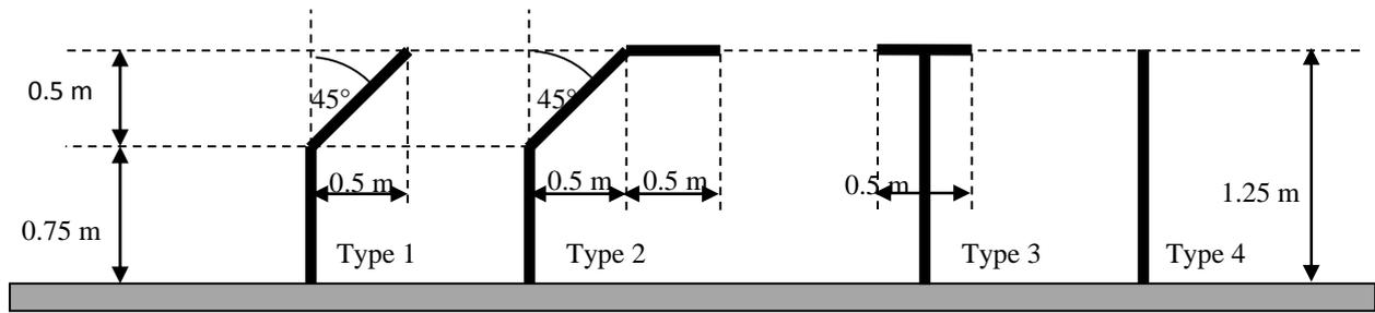
Fig. 1. Dimensions of the noise barriers for the measurements using scaled models
