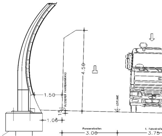
**Fig. 2.** Low and almost straight noise barrier
