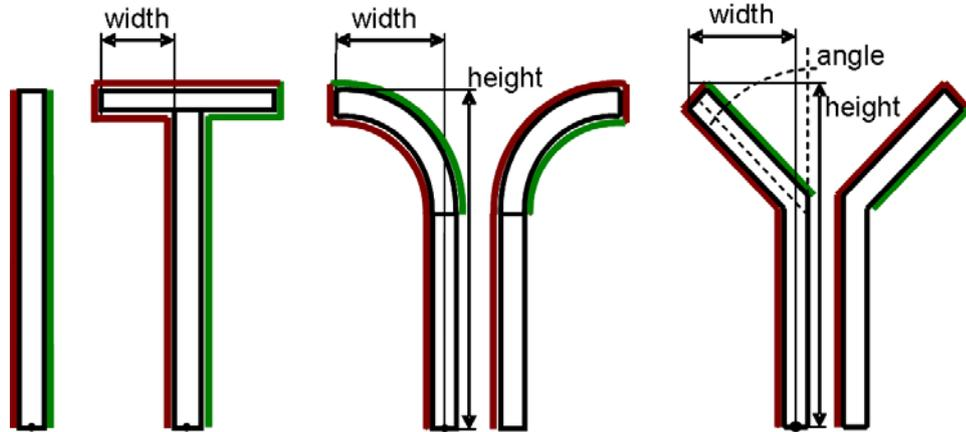
Fig. 5. Noise barrier types used in the simulation
