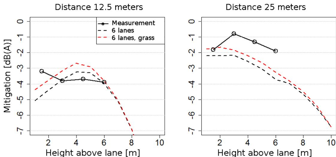
**Fig. 4.** In-situ validation results with and without a grassland model.
