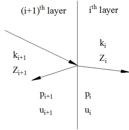
**Fig. 2.** Acoustic impedance and the wavenumber of bordering layers.
