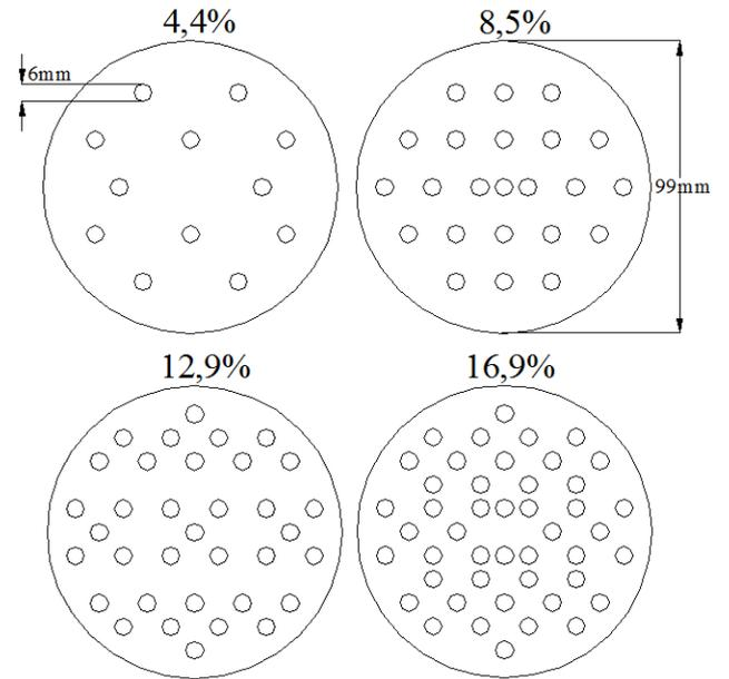
Fig. 3. Layout of perforated samples.
