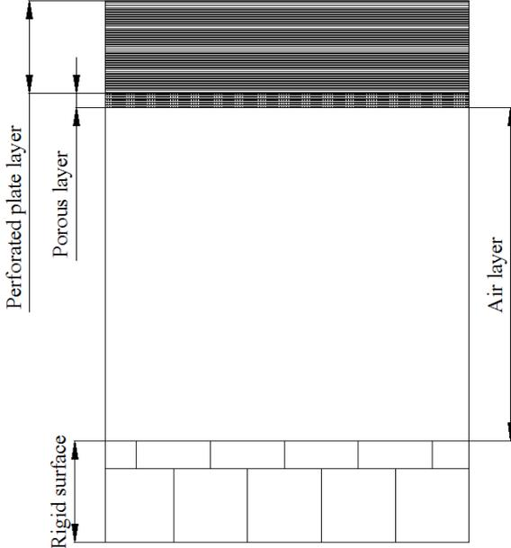
**Fig. 1.** Cross-section of the chosen setup.
