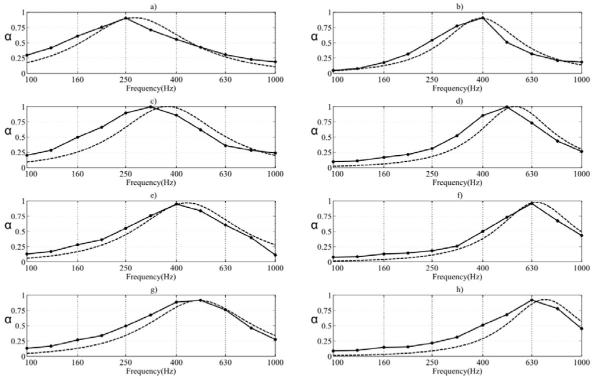
**Fig. 4.** Comparison of calculated and measured absorption coefficients. ——— measured, - - - - - calculated.
