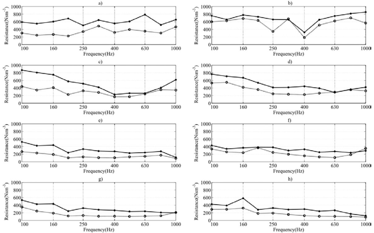
**Fig. 6.** Comparison of acoustic resistances of samples with tightly and loosely placed porous layers. ——— tight contact, ..... loose contact.
