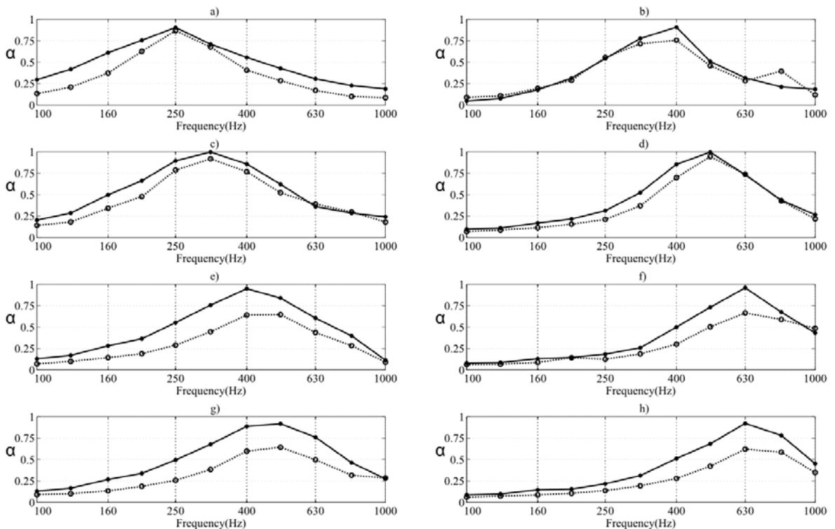
**Fig. 5.** Comparison of measured absorption of samples with tightly and loosely placed porous layers. ——— tight contact, ..... loose contact.
