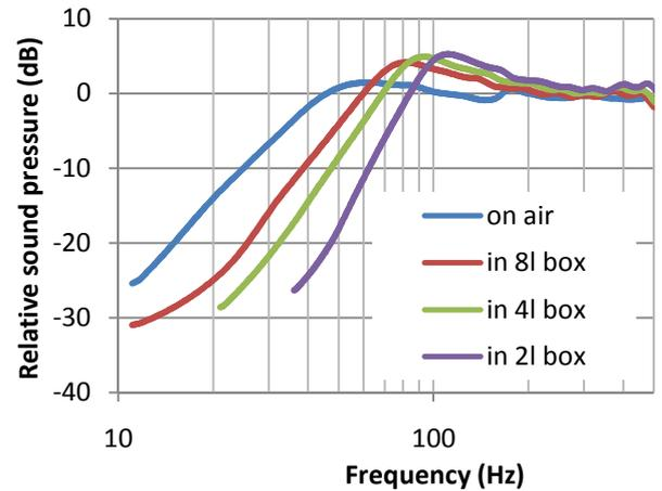
Fig. 9. Relationship between loudspeaker frequency response and box volume
