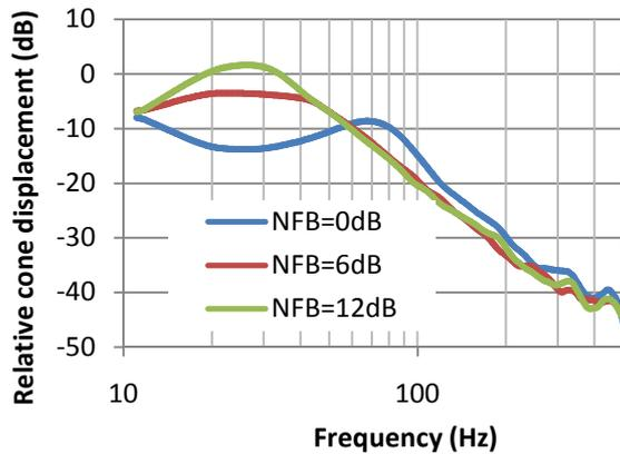
Fig. 11. Relationship between cone excursion and applied negative feedback
