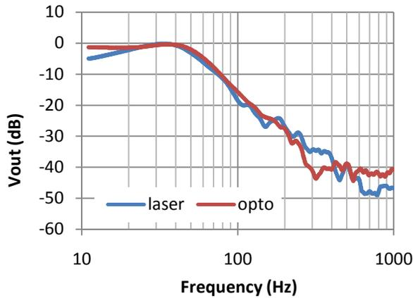
Fig. 7. Transfer functions of laser distance meter and optical position sensor
