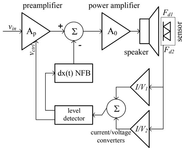
Fig. 4. Block-diagram of negative feedback implementation in active loudspeakers
