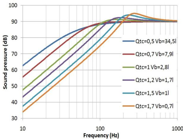
Fig. 2. Driver's transfer functions for different  $Q_{tc}$  and  $V_b$  values
