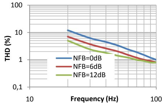
Fig. 13. Relationship between THD and applied negative feedback
