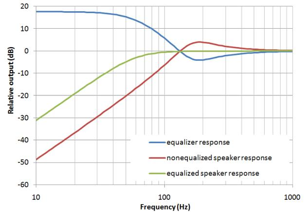
Fig. 3. Frequency responses of non-equalized driver, equalizer and equalized driver
