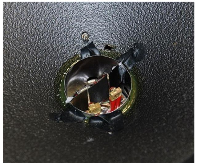
Fig. 6. Optical cone position sensor implementation
