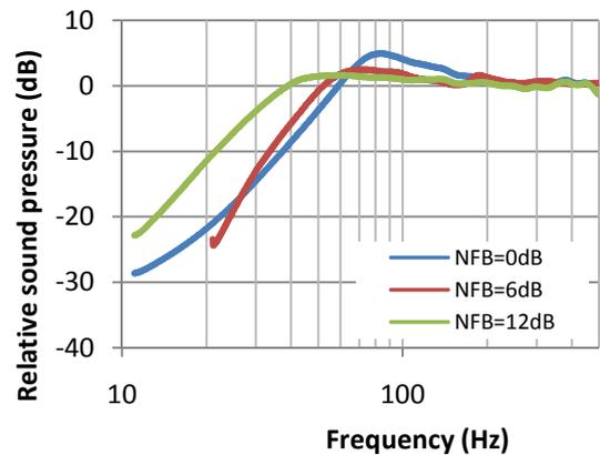
Fig. 10. Relationship between loudspeaker frequency response and applied negative feedback
