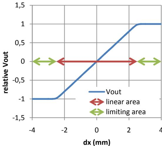
Fig. 5. Transfer function of preamplifier  $A_p$
