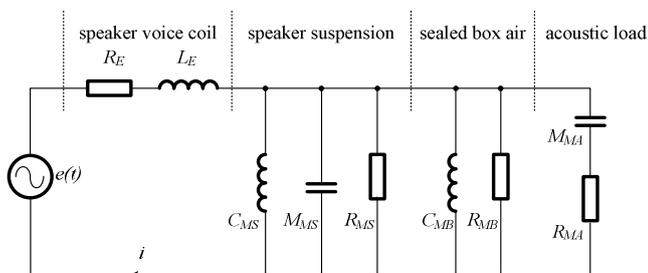
Fig. 1. Block-diagram of sealed-box woofer
