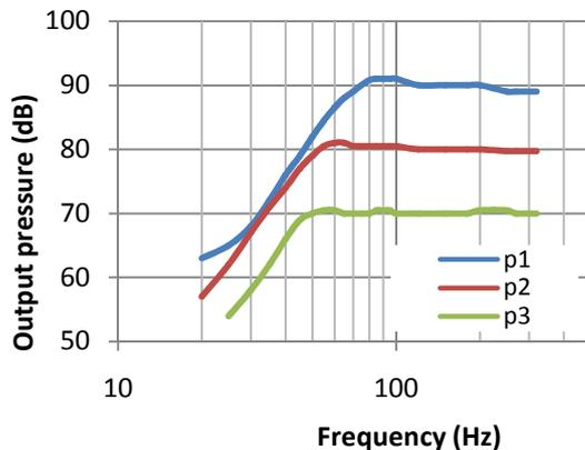
Fig. 12. Effect of cone over-excursion protection circuit
