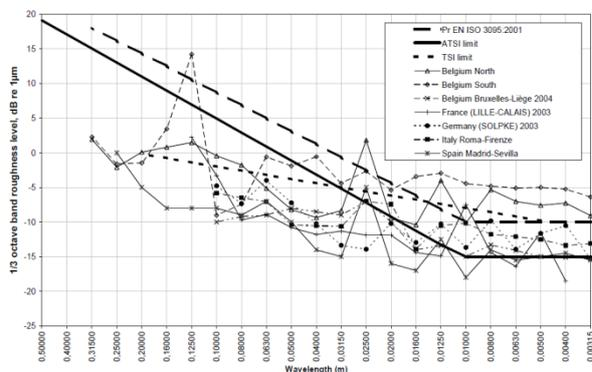
Fig.6. Measured rail roughness in the NOEMIE project
