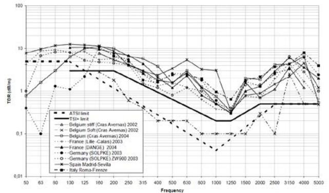
Fig.8. Measured lateral track decay rates in the NOEMIE project
