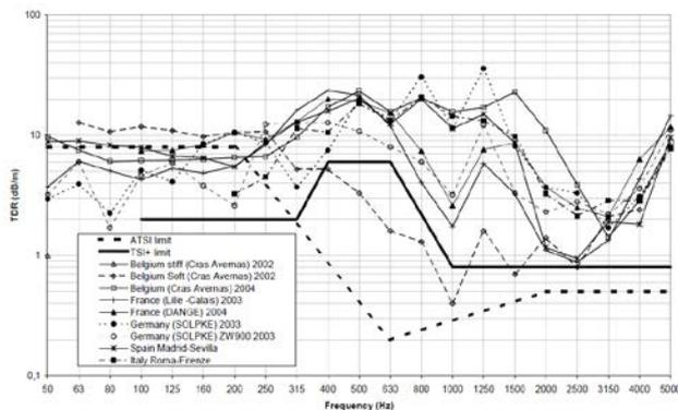
Fig.7. Measured vertical track decay rates in the NOEMIE project
