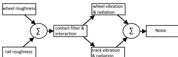
**Fig.3.** Model of rolling noise formation
