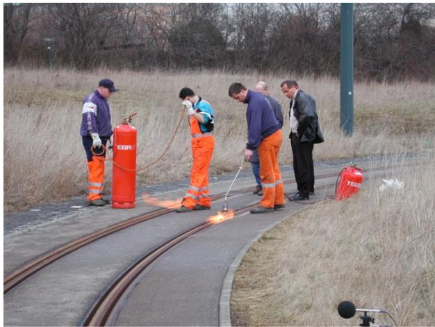
**Fig.2.** Heating up rails for squealing measurements
