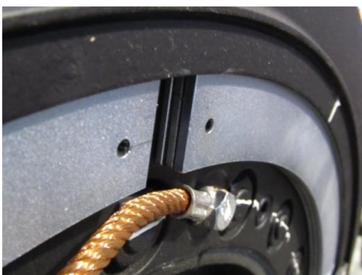
**Fig.10.** Examples of tramway wheel dampers
