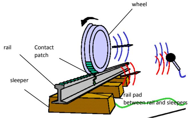
**Fig.4.** Illustration of rolling noise generation
