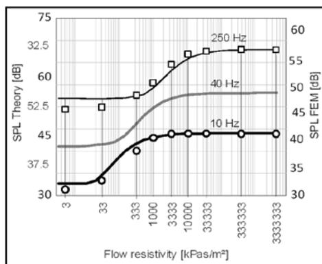
Fig.12. Correlation between sound pressure level at the observation point and flow resistivity of the sample
