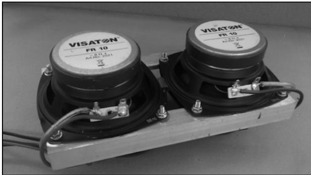
Fig. 2. A dipole configuration used for low frequency range
