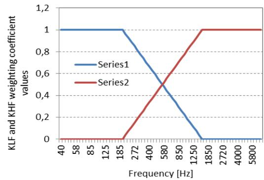
Fig.19. Weighting coefficients,  $K_{LF}$  blue curve and  $K_{HF}$  red curve
