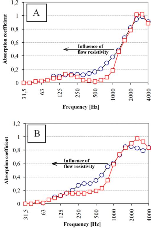
Fig. 8. Comparison of results; sound absorption coefficient measured in an impedance tube – blue curve, coefficient measured with a dipole in a Very Near Field – red curve. A: polyurethane foam, 10 mm thick, with density 60kg/m<sup>3</sup>, B: Polyurethane foam, 40 mm thick with density 50kg/m<sup>3</sup>
