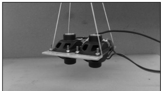
Fig. 4. A dipole used for high frequency range
