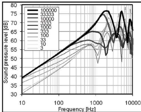
Fig.11.Sound pressure at point  $p$  obtained with FEM analysis
