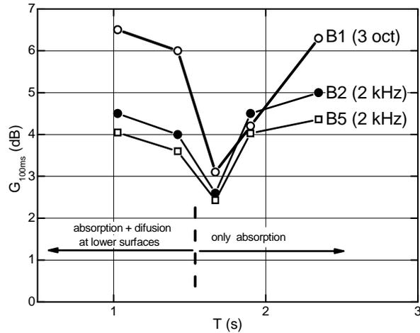
Fig.10 Three examples of gain variation as a function of reverberation time in the hall
