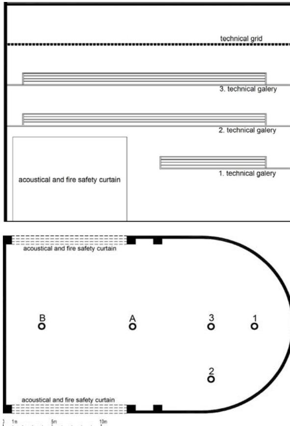
Fig.2 Base and crosssection of the analysed hall; the positions of sound source (A and B) and receiver (1,2 and 3) used in the analysis are marked at the hall base.
