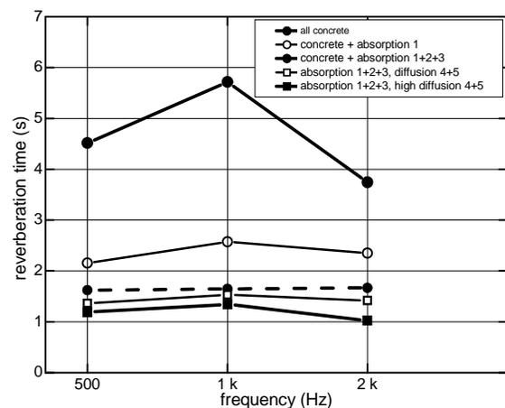
Fig. 6 The results of reverberation time measurements
