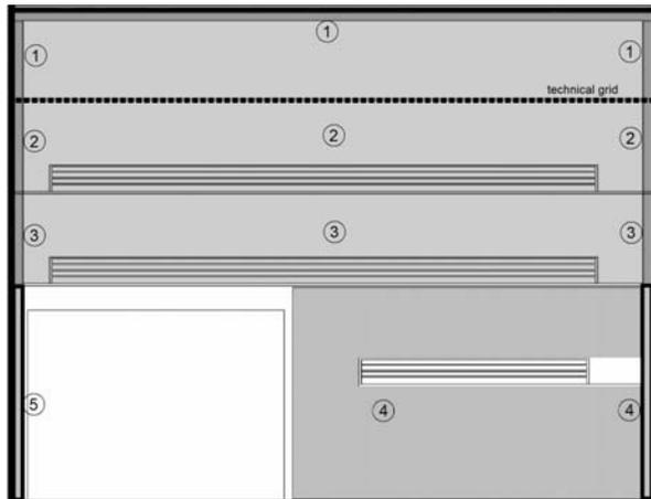
Fig. 3 The schematic presentation of acoustics interventions in the hall: 1, 2 and 3 - high efficiency absorbing material, 4 and 5 - relief that may be normal or complex (lower and higher value of scattering coefficient)
