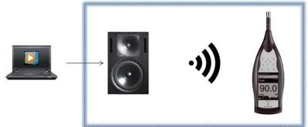
Fig. 1. Calibration of the system for subjective testing
