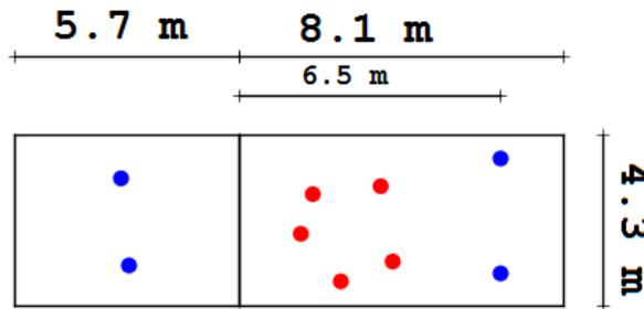
**Fig.2.** Microphone (blue dots) and sound source (red dots) positions in the source (right) and receiving rooms (left) as proposed by the impulsive method. Room dimensions are also shown.
