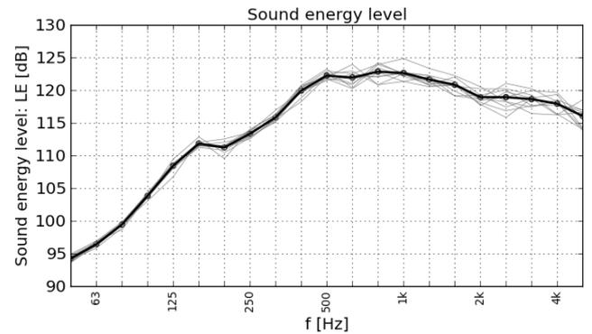
**Fig.1.** One third octave spectrum of sound energy level of gunshot (gray curves-individual measurements, black curve - average value).
