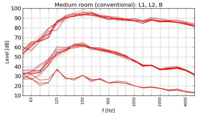
**Fig.8.** Averaged sound pressure levels as measured in the source and the receiving room by the conventional method. Dotted lines represent measurements when sound source in the sourceroom was at the first position, while full lines represent measurements when sound source was at the second position.
