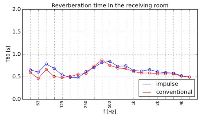
**Fig.4.** Reverberation time in the receiving room as measured by the conventional (red line) and impulsive (blue line) method.
