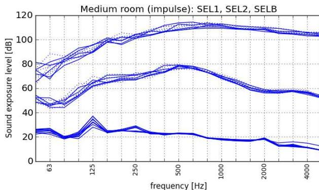
**Fig.3.** Sound exposure level measurements in the source ( $SEL_1$ ) and receiving rooms ( $SEL_2$ ) with background noise
