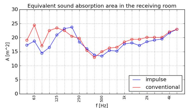
**Fig.5.** Equivalent sound absorption area in the receiving room as measured by the conventional (red line) and impulsive (blue line) method.
