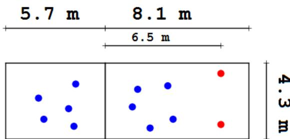
**Fig.7.** Microphone (blue dots) and sound source (red dots) positions in the source and receiving rooms as proposed by conventional method [1]. Five microphone positions were chosen in each room separated by common partition. Two sound source positions were chosen opposite common wall. The dimensions of both rooms are also shown.
