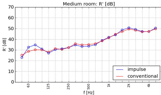
**Fig.6.** Apparent sound reduction index of common lightweight partition between two medium sized rooms.
