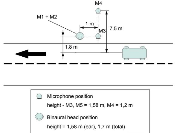
**Figure 1:** measurement setup for the investigated traffic scenarios of a pass-by situation
