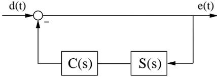
**Fig. 1.** Block diagram of the closed feedback loop, where  $C(s)$  describes the filter to shape  $S(s)$  (i.e. the secondary path) to form an stable closed loop.
