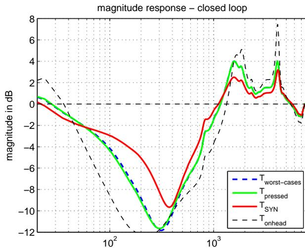
**Fig. 5.** Performance analysis of 2nd order optimal filters applied to the pressed secondary path. The filter  $C_{\text{onhead}}$  designed only for the standard wearing situation violates the design constraint (i.e.  $20 \log \max |T(s)| \leq 4\text{dB}$ ).
