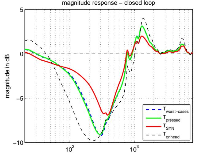
**Fig. 4.** Performance analysis of 2nd order optimal filters in Fig. 3 applied to the nominal secondary path (i.e standard fitting of the headphone). The design constraint for the maximum amplification restricts the magnitude to be smaller or at least equal to 4dB.
