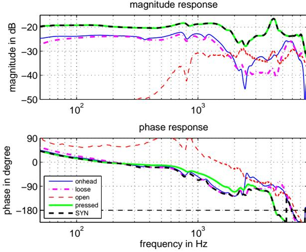
**Fig. 2.** Measurement scenarios: The case when the headphone is pressed against the ear yields a frequency response with the largest magnitude and a fast falling phase. The opposite result is seen when the headphone is not put on (open). It is not possible to use only one measurement to define an overall worst-case, although we can construct a synthesized frequency response out of the worst-case pieces of all measurements (SYN).
