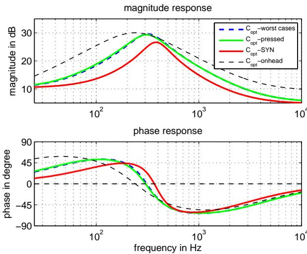
**Fig. 3.** Outcome of the optimization for 2nd order optimal filters with different secondary paths in the constraining function. Synthesized constraints result in the most conservative optimal filter, whereas an optimization on the nominal secondary path leads to the opposite.
