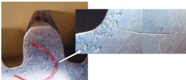
**Fig. 2.** Pinion with a fatigue crack in the tooth root [1]
