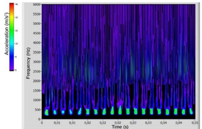
**Fig. 3.** Frequency scalogram of wavelet coefficient of the reference gear unit
