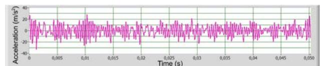
**Fig. 9.** Measured signal of vibrations of a gear with a pinion with a crack
