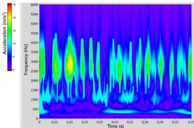
**Fig. 6.** Frequency scalogram of square wavelet coefficient of the gear unit with a crack in a tooth root
