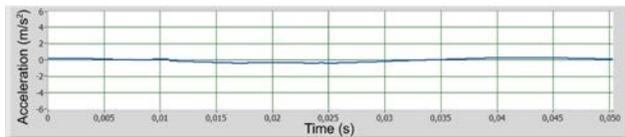
**Fig. 10.** With Morlet wavelet de-noised signal of vibrations of a faultless gear unit
