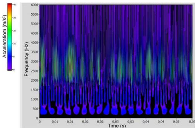
**Fig. 5.** Frequency scalogram of wavelet coefficient of the gear unit with a crack in a tooth root
