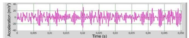
**Fig. 8.** Measured signal of vibrations of a faultless gear unit
