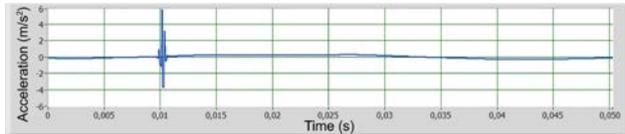
**Fig. 11.** With Morlet wavelet de-noised signal of vibrations of a gear with a pinion with a crack
