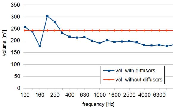
Figure 6: The reduced volume of the reverberation chamber
