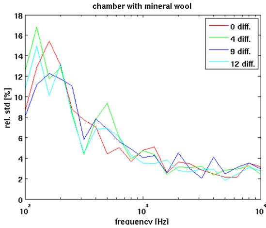
Figure 4: std. of  $R_T$  with 0, 4, 9, 12 diffusors, with mineral wool
