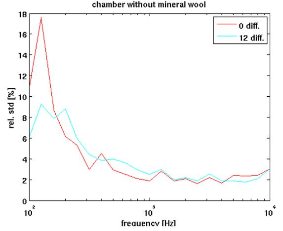
Figure 1: Standard deviation of  $R_T$  with 0 and 12 diffusors
