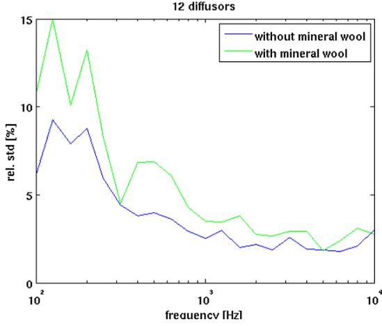
Figure 3: std. of  $R_T$  with 12 diffusors, with and without mineral wool
