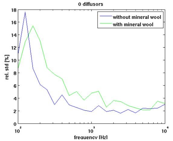
Figure 2: std. of  $R_T$  with 0 diffusors, with and without mineral wool
