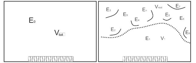
Figure 5: Energy density distribution without and with diffusors
